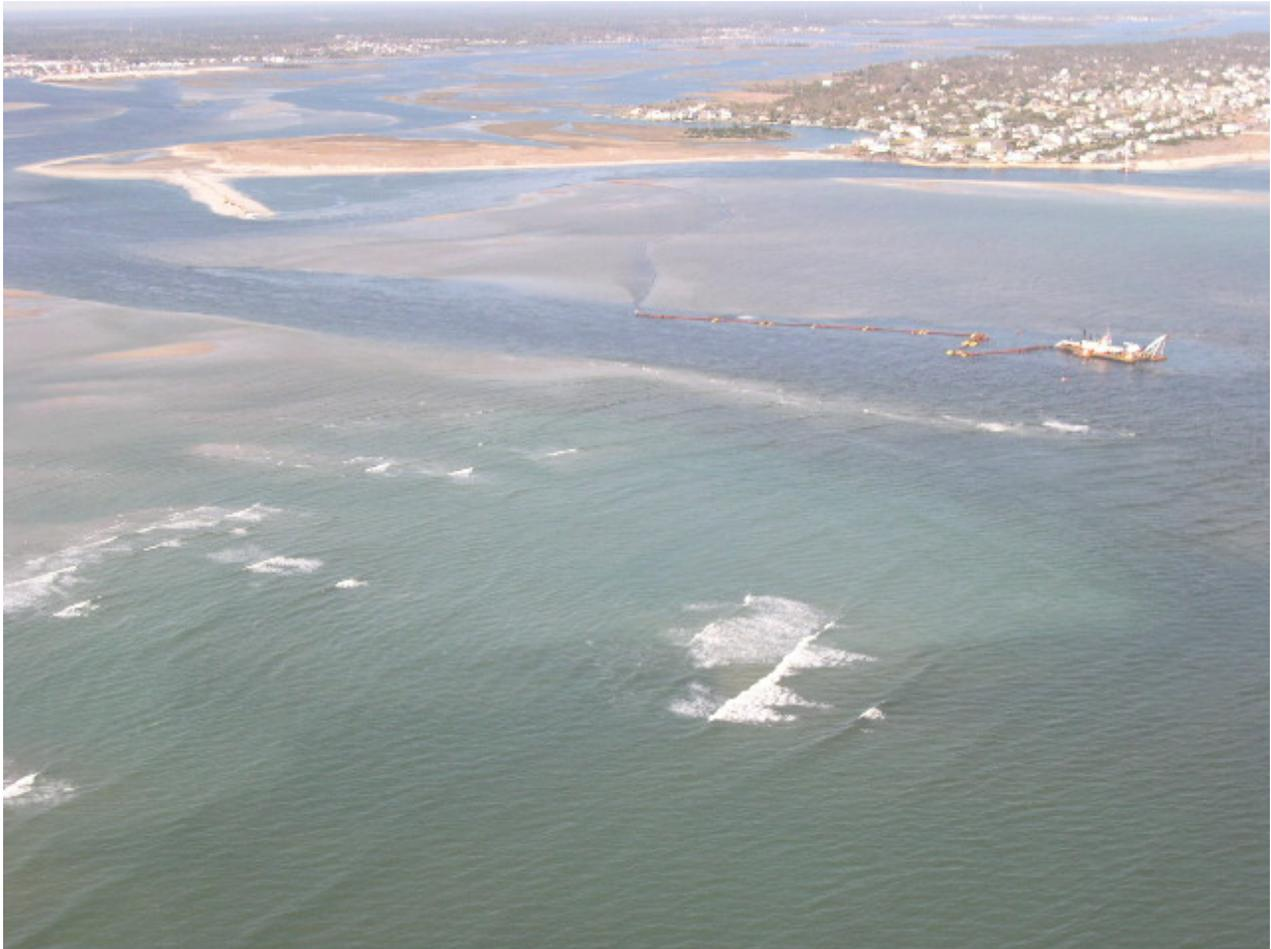
The picture above was taken on April 11, 2005, approximately 11 days prior to full project completion. The dike shown in the picture above is approximately 1,300 feet long, and was eventually extended to a total length of 2,200 feet when the project was completed on April 22. The dike ties into the existing shoals shown in the photo above, and prevents flow into the old channel in Bogue Inlet. (Photo courtesy of Carteret County Shore Protection Office.)
