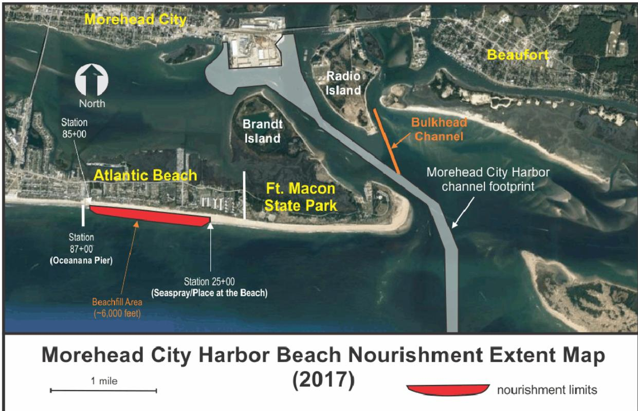
Fig. 2 – Site map depicting the general footprint of the Morehead City Harbor Federal Navigation Project and beach placement zone of dredged material associated with the Spring 2017 Outer Harbor maintenance event.
